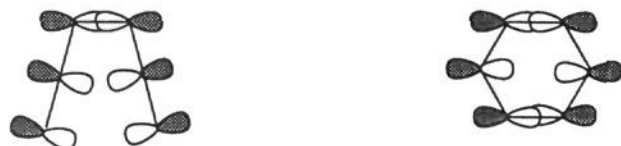
Figure 3. In-plane 2p orbitals of (left) hex-3-ene-1,5-diyne and (right) the singlet p -benzyne biradical, which were chosen to be active in the CASSCF calculation of this study.
